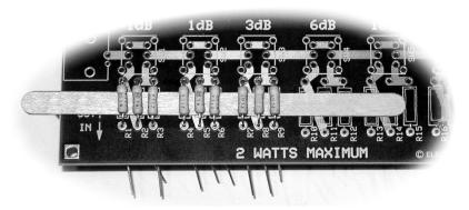
Figure 2. Spacing Resistors Above the Board.
