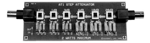
Figure 1. Assembled AT1 Step Attenuator.
